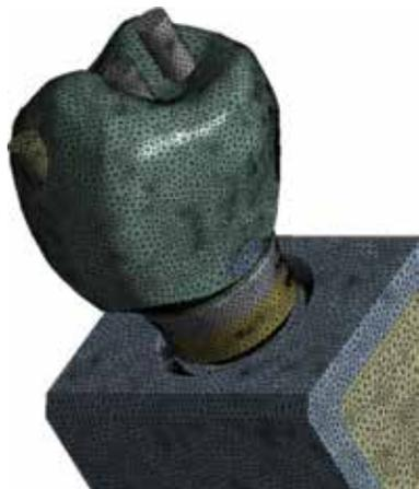
Figure 7. Mesh of the finite element model.
