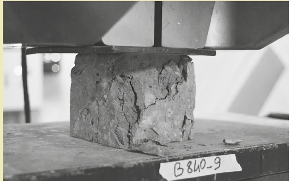
Compression of adobe sample mixed with bamboo powder Source: Authors' photo.
