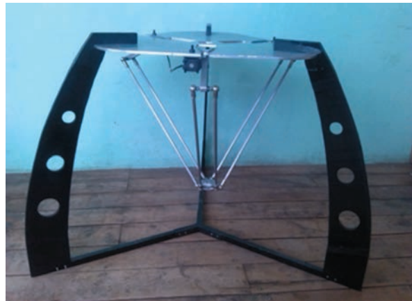
Fig. 1. SCHEME OF THE USED DELTA ROBOT
