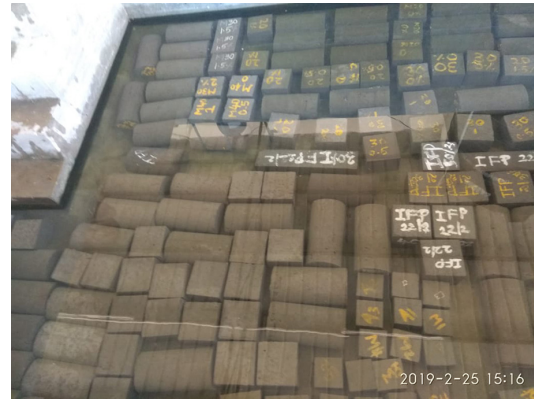
Fig. 3. SPECIMENS UNDER CURING FOR ALL CONCRETE MIX DESIGN
