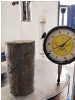
Fig. 2. SOIL SAMPLE DURING UCS TESTING
