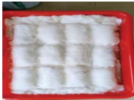
Fig. 5. SAMPLES FOR DURABILITY TEST UNDER WETTING AND DRYING CYCLES
