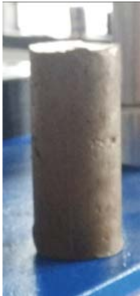
Fig. 1. SOIL SAMPLE PREPARED FOR UCS TESTING
