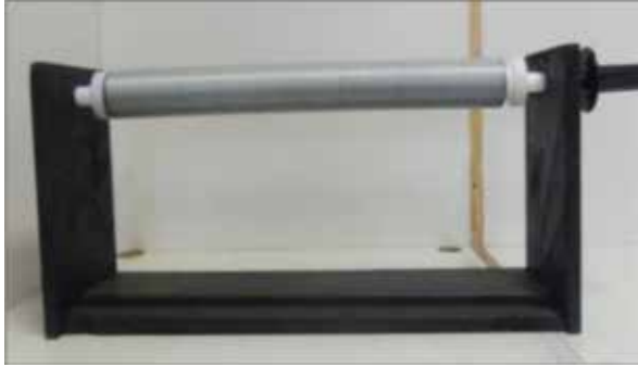
Fig. 3. WINDING OF NYLON/EPOXY EXTERNAL LAYER
