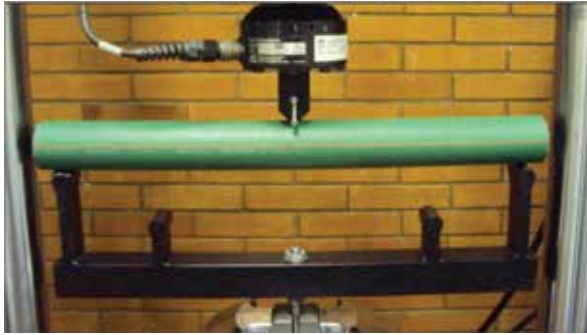
Fig. 4. TEST SETUP FOR THE CIRCULAR BEAMS
