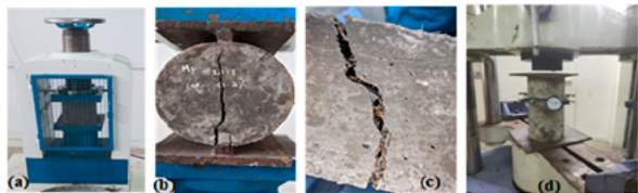
Fig.3 EXPERIMENT TEST SETUP (a) COMPRESSION (b) SPLIT TENSILE (c) FLEXURE (d) MODULUS OF ELASTICITY
