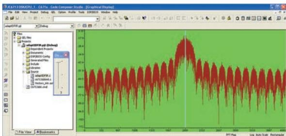
a) FFT Applied to Desired Signal (BandPass FIR Filter Response)
