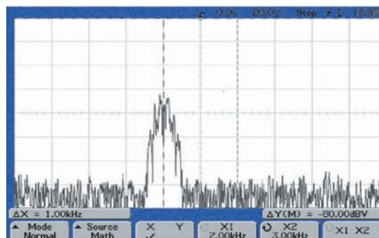
a) FFT applied to desired signal
