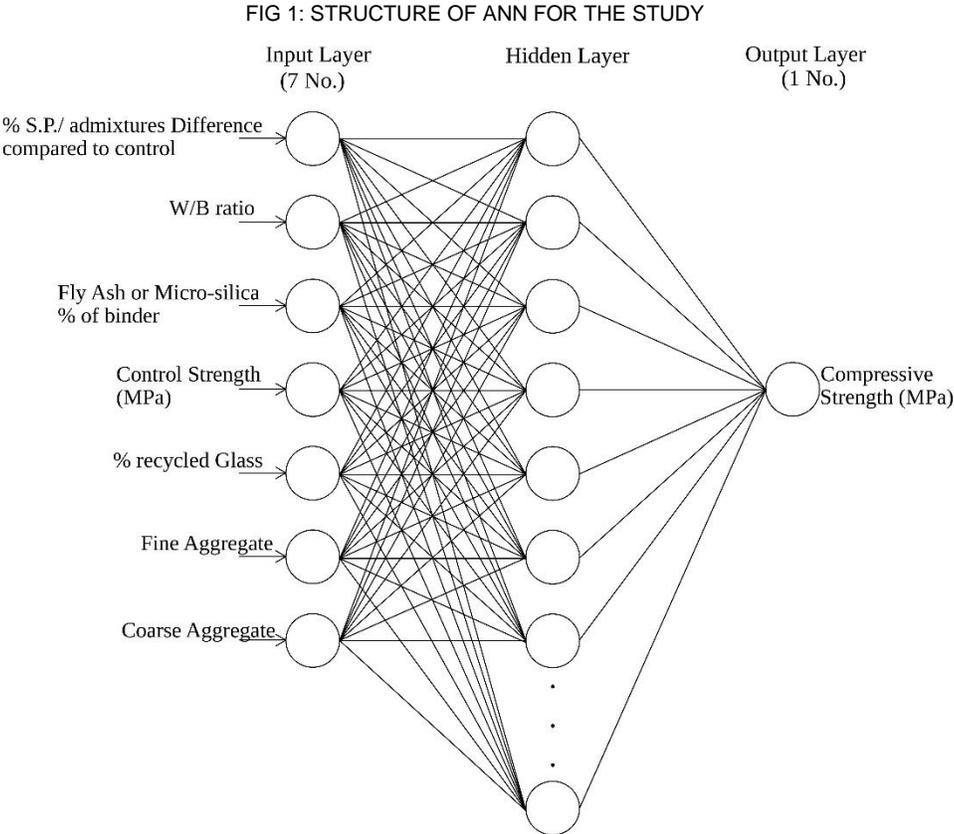
The structure for ANN models was developed and run in GNU Octave. According to Eaton *et al.* [7], GNU Octave is a high-level language to solve problems such as linear and non-linear equations and statistical analysis and other numerical experiments. The network was developed based on Oman [22] illustration on neural network using Octave. According to Oman [22], back propagation algorithm goal is to train the network to minimize cost, with the error at a certain layer in the network taken and
